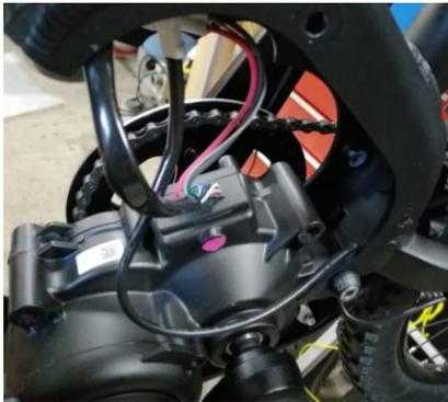
*Fig. 4 Loosening the motor*
