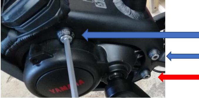
*Fig. 3 Loosening the motor*
