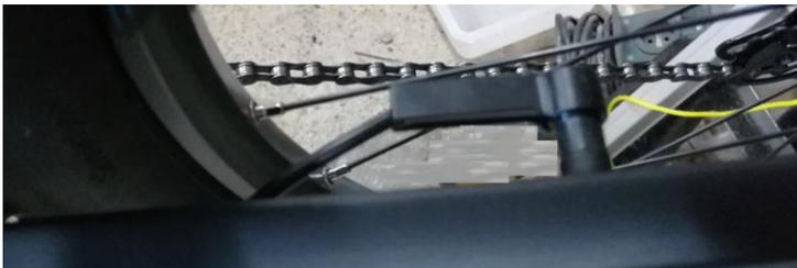
*Fig. 1 Speed sensor*
