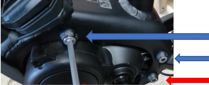
*Fig. 3 Loosening the motor example (motor / manufacturer may differ)*
