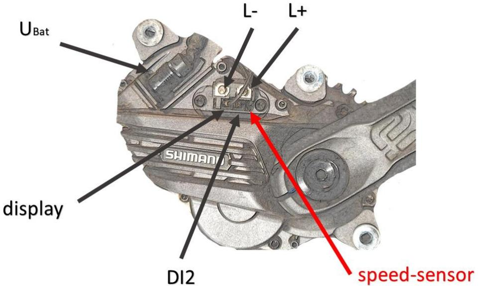
Fig. 2 Connector end of the speed sensor
